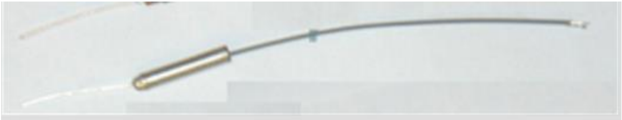
Figure 3. HF-LPB125 外置天线接头示意
